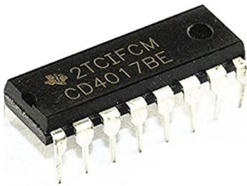
Figure 4: CD4017 IC & Pin Configuration.
